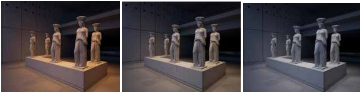
Figure 2: Real-time simulated space with different correlated color temperature (CCT): 2700K (left), 4000K (centre) and 6000K (right)
